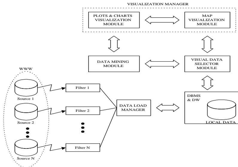
**Fig. 2.** The SEISMO-SURFER architecture.
